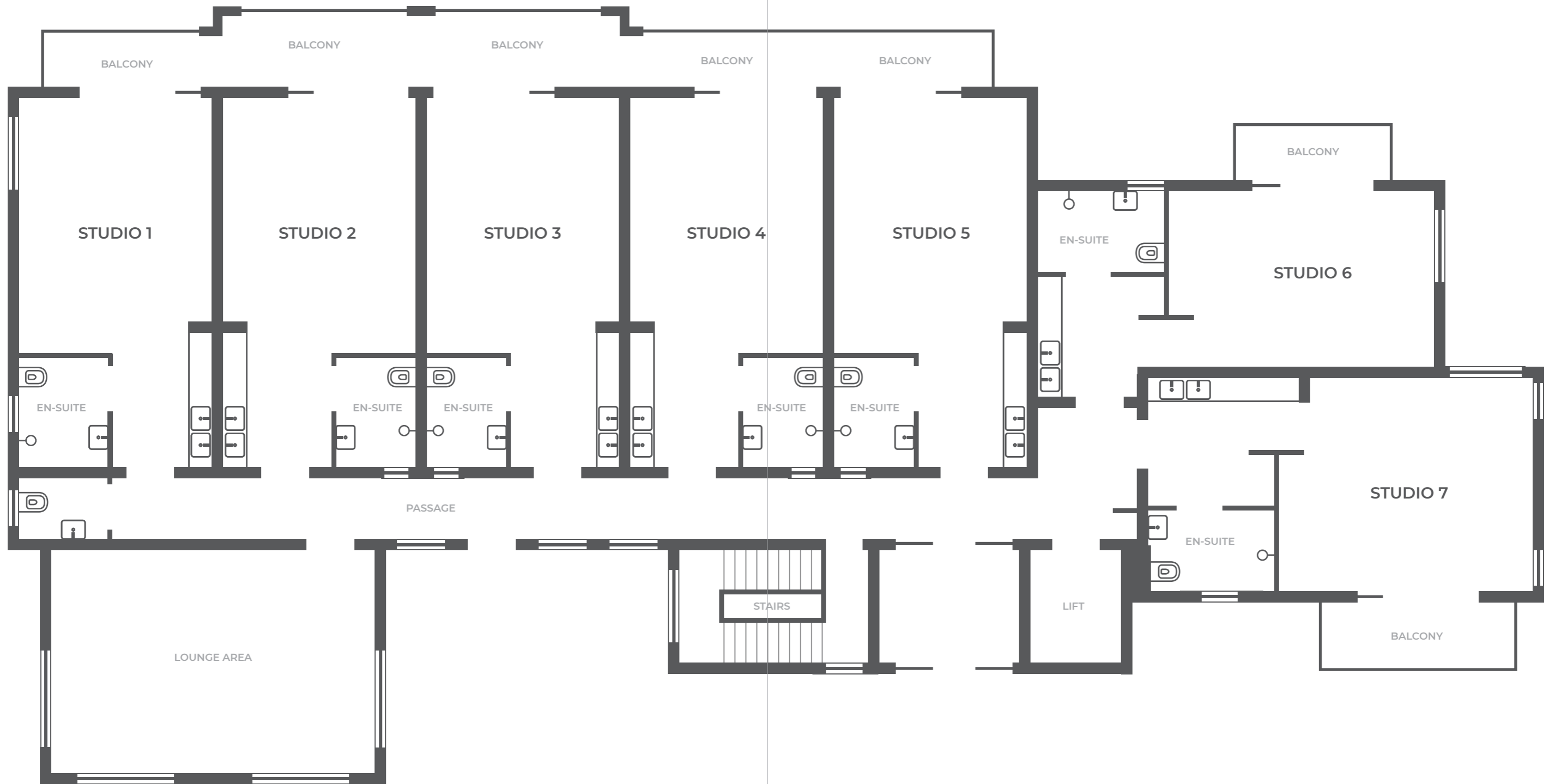
LARMENIER CARE CENTRE BUILDING 1 – FIRST FLOOR PLAN
